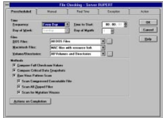
Another of the File Checking pages: the Prescheduled option allows the administrator to configure when and what to scan.
